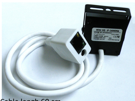
Cable length 60 cm No connector on the camera rear face
