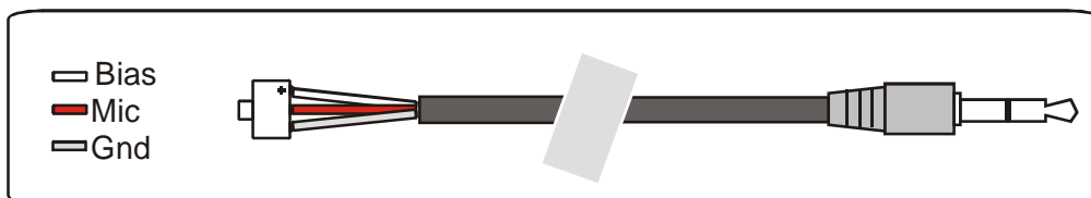
Figure 4: Example Wiring to Knowles EA Series Microphones
