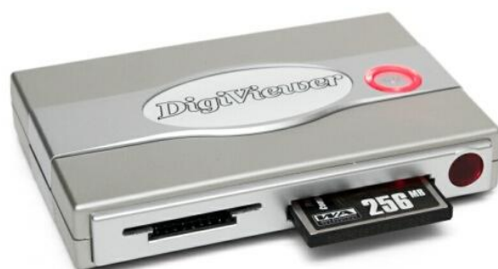
Figure 13: DigiViewer for Playing FlashBack Recordings to a TV Monitor
